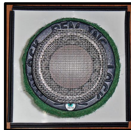
Mesh Top Covering Overflow Port
