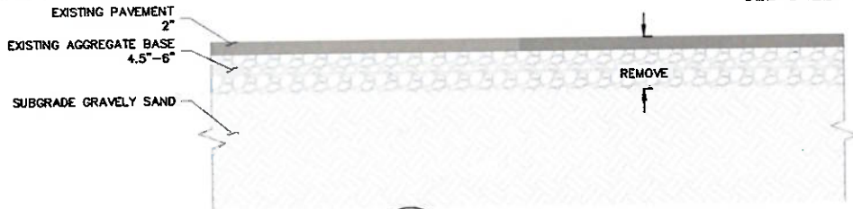
A EXISTING AC PAVEMENT SECTION SCALE: NTS
