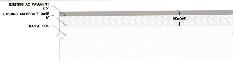
A EXISTING AC PAVEMENT SECTION (CL-01) SCALE: 1"=1'
