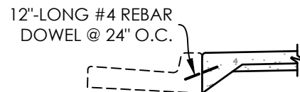
CURB-TO-SIDEWALK DOWELING SEE NOTE 2
