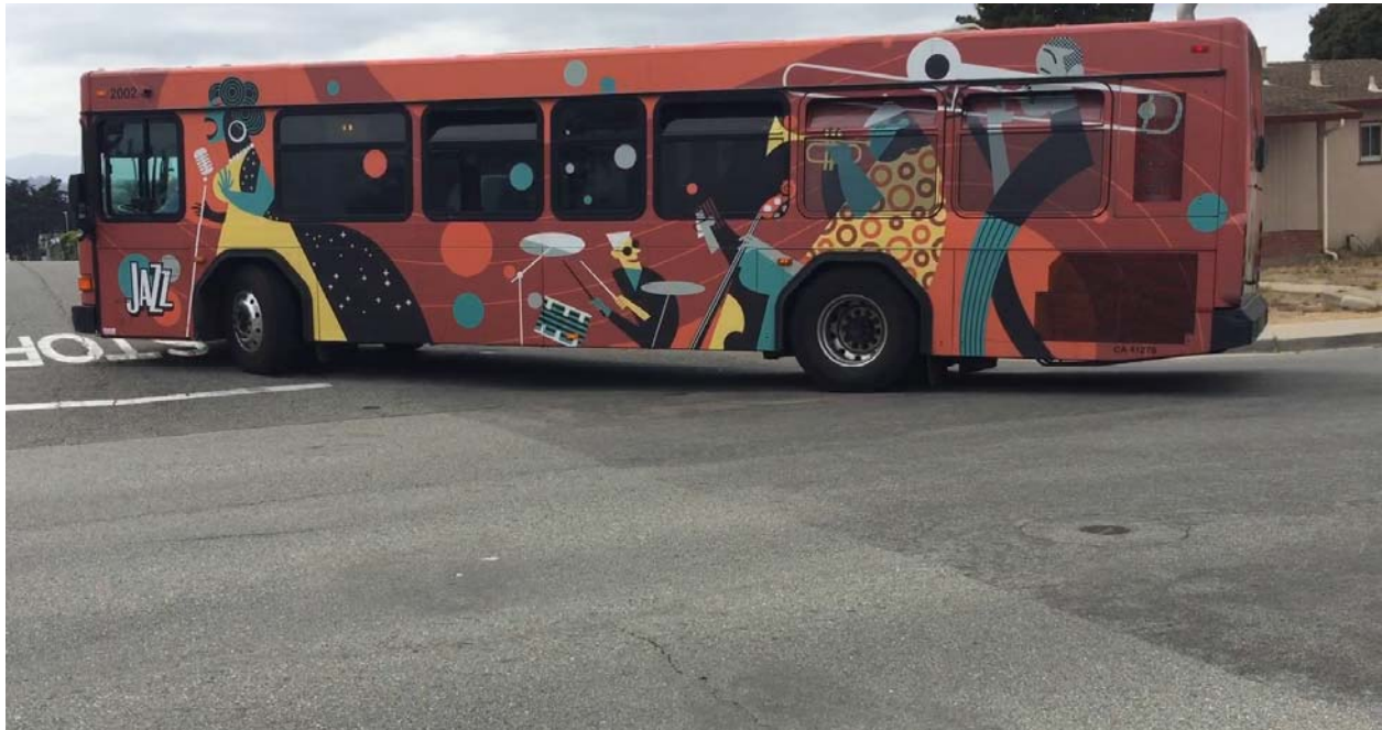
MST turning onto SB Flores St from La Salle with vehicles parked on the corner. Picture shows MST encroaching onto NB lane on Flores Street.
