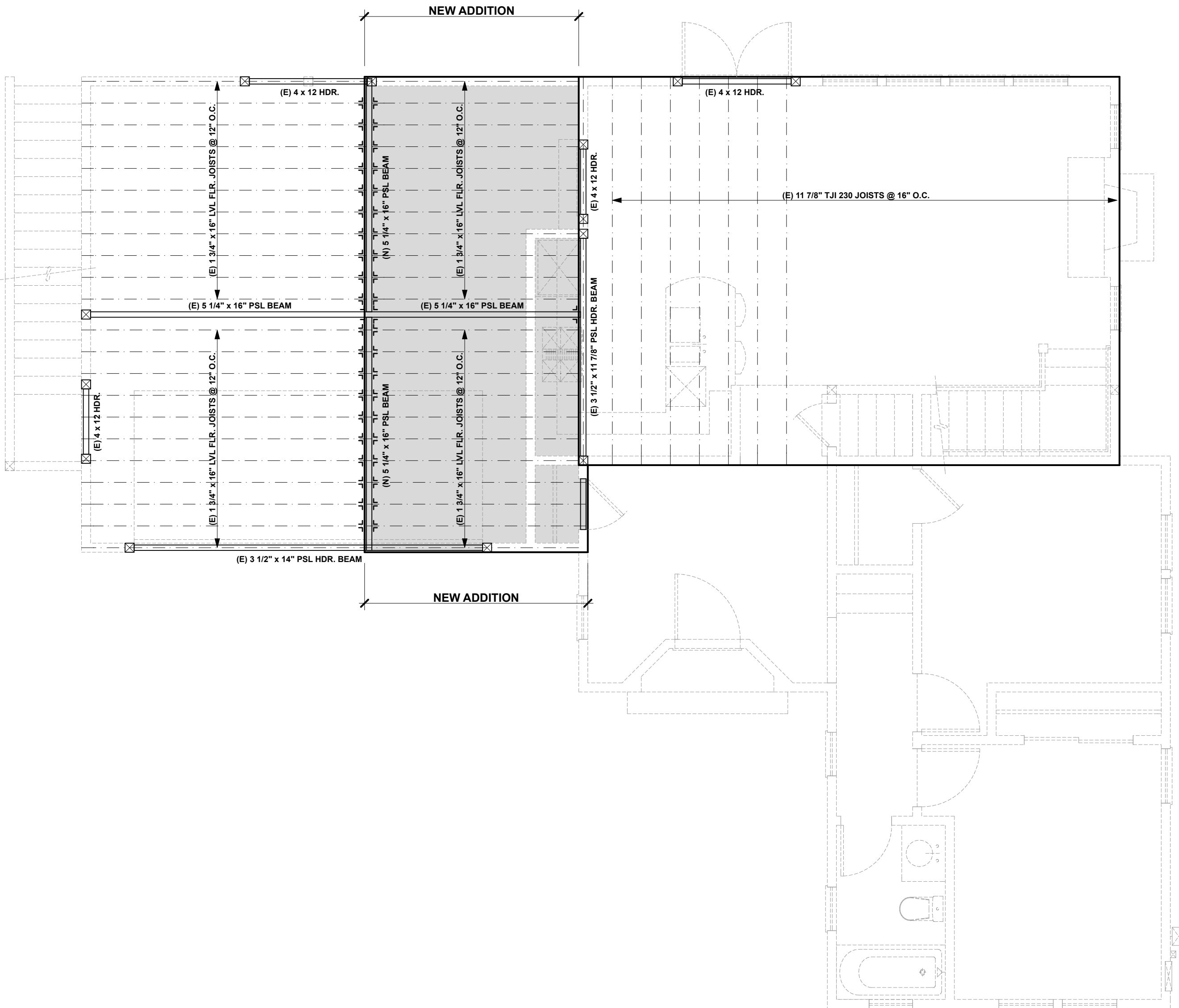
Upper Floor Framing Plan 1/4" = 1'-0"
