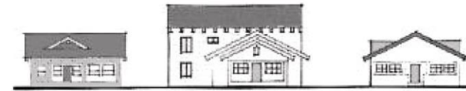
Inappropriate Usage of Mass and Scale.
